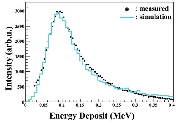
Fig. 2. Energy deposit distribution of the first layer for  $\beta$ -rays from the  $^{90}\text{Sr}/^{90}\text{Y}$  source.
