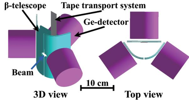
Fig. 1. Schematic view of the detector system.
