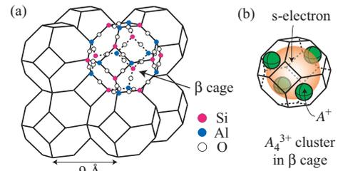
Fig. 1. Schematic illustrations of (a) the crystal structure of sodalite and (b) the  $A_4^{3+}$  cluster formed in the  $\beta$  cage, where  $A$  indicates an alkali element.
