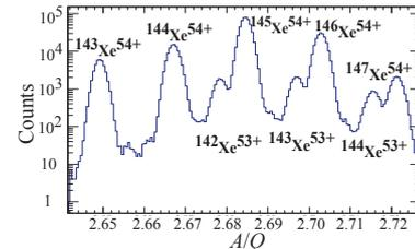
Fig. 1.  $A/Q$  spectrum of neutron-rich Xe isotopes.
