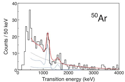
Fig. 2. (colour online) Doppler-corrected  $\gamma$ -ray energy spectrum for  $^{50}\text{Ar}$ . The black dotted line and the blue dashed lines are an exponential fit to the background and GEANT4 simulations, respectively; the solid red line is the total (sum) fit.
