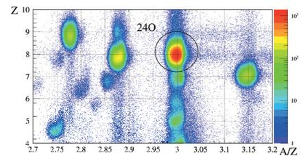
Fig. 1. PID plot of the <sup>24</sup>O beam setting
