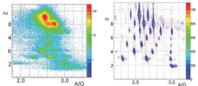
Fig. 2. Z vs A/Q plots under beam trigger; (left) downstream; (right) upstream.
