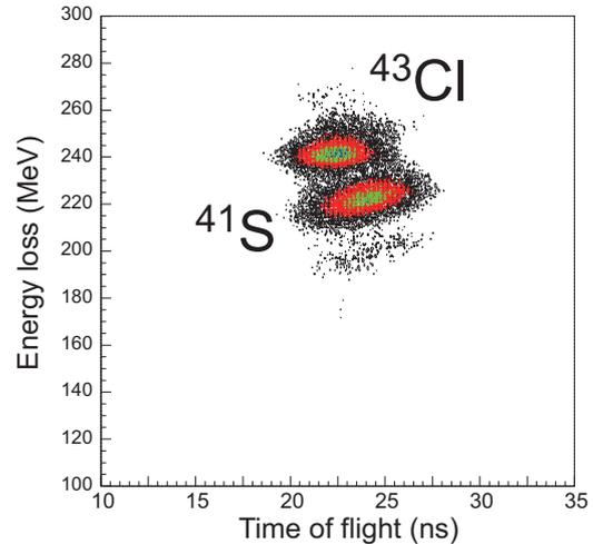
Fig. 1. Particle identification of  $^{41}\text{S}$ . The horizontal and vertical axes represent TOF between the plastic scintillators at F2 and F3, and  $\Delta E$  taken at the silicon detector at F2, respectively.
