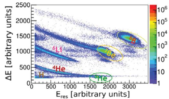
Fig. 1.  $\Delta E$ - $E_{\text{res}}$  identification of the different ions produced in the scattering of the cocktail  $^8\text{B}$ - $^7\text{Be}$ - $^3\text{He}$  beam onto a  $^{208}\text{Pb}$  target.
