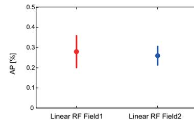
Fig. 2. Obtained  $A_\beta P$  value of  $^{20}\text{F}$  with applied linear RF field.
