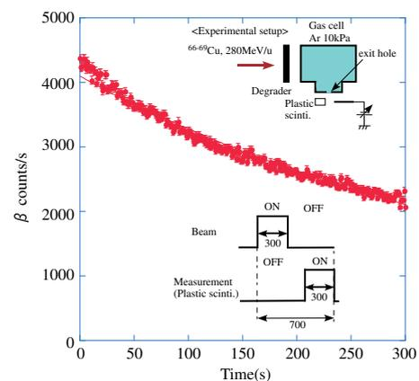
Fig. 2. Beta ray counts of the extracted RIs.
