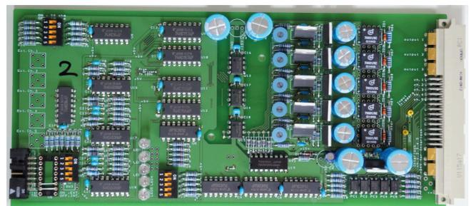
Fig. 2. Photo of the timing-controller circuit board. The left side is for the external trigger input area, and the right internal. The black connector at the left bottom is selector pins for the int./ext. input switches.
