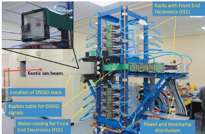
Fig. 1: A photograph of the fully constructed AIDA assembly.
