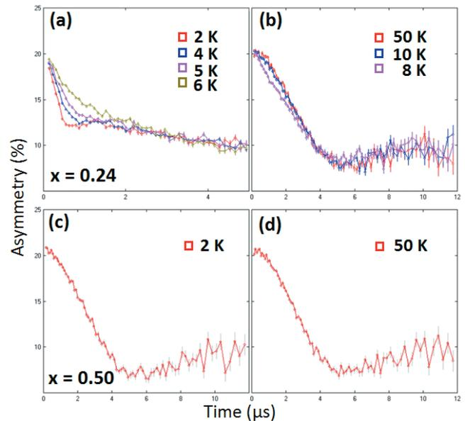
Fig. 2 ZF- $\mu$ SR of  $\text{Ce}_{1-x}\text{La}_x\text{Os}_2\text{Al}_{10}$
