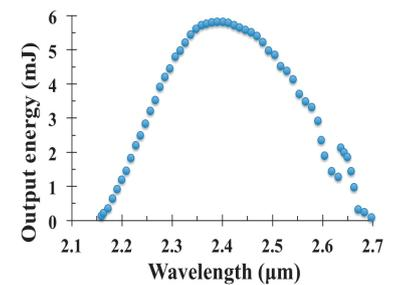
Fig. 2. Output energy of the for Cr:ZnSe laser
