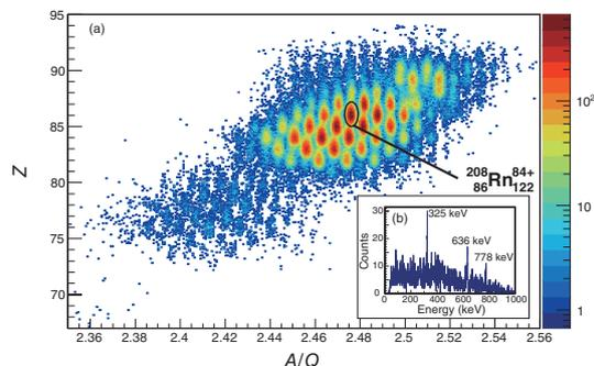
Fig. 1. (a) Particle identification plot for the RI beam measured at the second stage of BigRIPS. The atomic number  $Z$  versus the mass to charge ratio is shown. (b) The  $\gamma$ -ray energy spectrum of the known isomeric state in  $^{208}\text{Rn}$ , indicated by the circle in (a). Three  $\gamma$ -ray peaks can be clearly observed.
