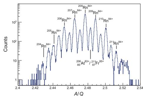
Fig. 2. Mass to charge ratio of the radon isotope ( $Z = 86$ ) obtained from Fig. 1 (a) with the gate of  $85.8 < Z < 86.2$ . The radon isotopes with  $Q = 84$  were observed between the masses 204 and 211, as can be seen for the isotopes labeled using lines.  $^{206}\text{At}^{83+}/^{211}\text{Fr}^{85+}$  shows a typical example of the contaminants for isotopes with  $Z = 85$  and  $87$ .
