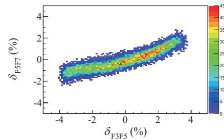
Fig. 2. Results of the momentum compression at the second stage of BigRIPS.  $\delta_{F3F5}$  and  $\delta_{F5F7}$  are  $(p - p_0)/p_0$  before and after using the momentum-compressive degrader, where  $p$  is the momentum and  $p_0$  is the momentum at the central trajectory.
