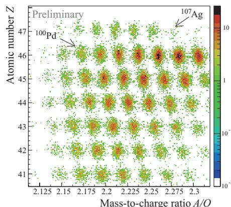
Fig. 1. Particle identification plot of  $Z$  versus  $A/Q$  in the ZeroDegree spectrometer for the reaction residues produced from the <sup>107</sup>Pd beam at 220 MeV/nucleon.
