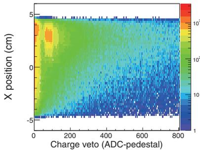
Fig. 1. The charge distribution in the CV vs the  $x$  position measured by the SMD for  $p+p$  from 2008 data. One MIP peak around the 100 ADC value in the positive  $x$  region, where the proton beam bending direction, is shown.
