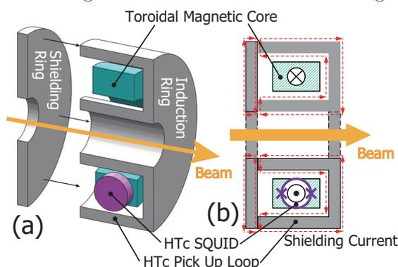
Fig. 1. New scheme of a HTc SQUID monitor.
