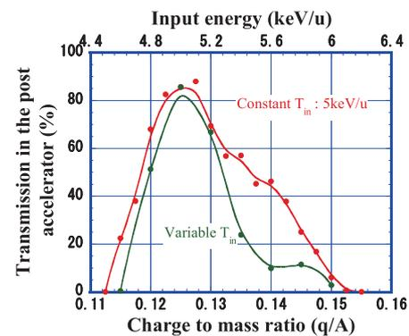
Fig. 2. The  $q/A$  dependence of the transmission.
