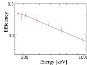
Fig. 1. Absolute  $\gamma$ -ray efficiency of EURICA.
