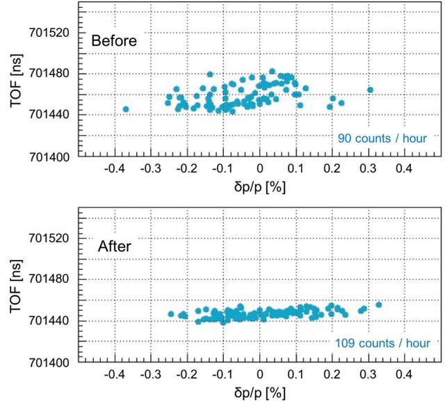
Fig. 2. TOF spectra of <sup>78</sup>Ge after extraction as a function of momentum. Upper and lower figures show the results obtained before and after adjusting the isochronism by the second order, respectively.
