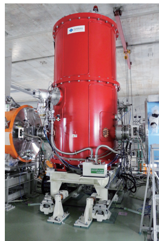
Fig. 2. A photograph of the delivered RF deflector.
