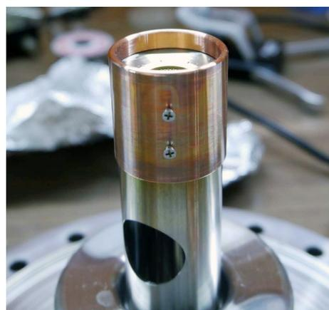
Fig. 2. Photograph of electron gun. The top copper sleeve is the newly installed part for concave equipotential surface to generate a focused electron beam.
