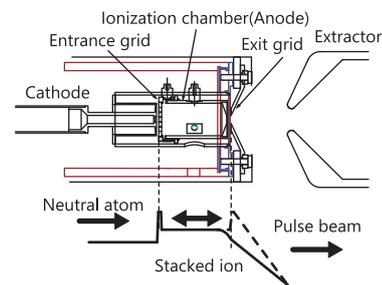
Fig. 1. Schematic drawing of the new ionization chamber of the ERIS. The schematic potential structure is also shown.
