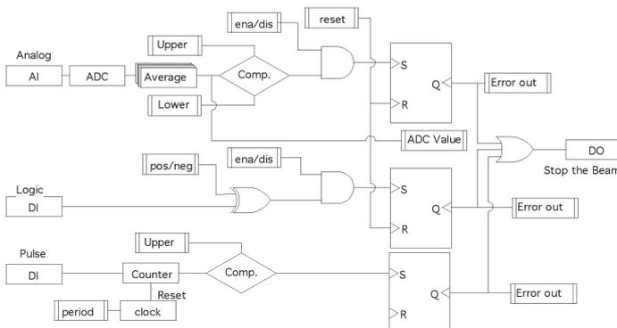
Fig. 1 Logic diagram of the fast beam interlock system.
