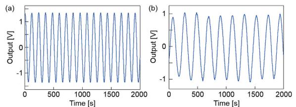
Fig. 1. Maser signals obtained for (a)  $^{129}\text{Xe}$  and (b)  $^{131}\text{Xe}$ . Beat signals from the lock-in amplifiers which were employed to improve the signal-to-noise ratio were observed at the reference frequency of 33.036 Hz for  $^{129}\text{Xe}$  and 9.797 Hz for  $^{131}\text{Xe}$ .
