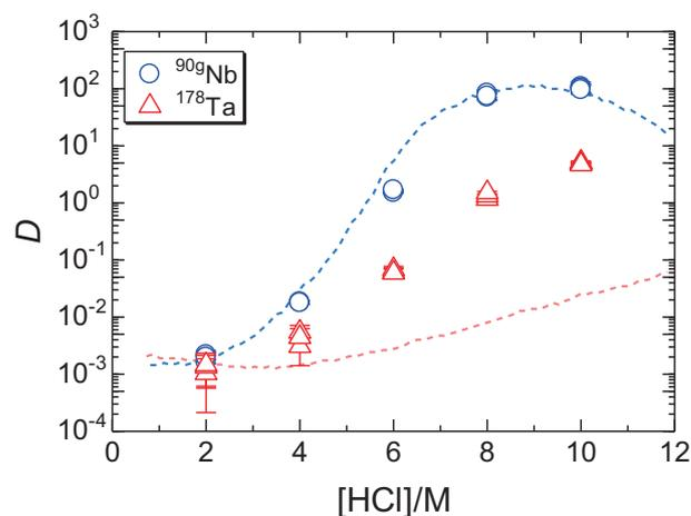
Fig. 1. Distribution ratios of <sup>90g</sup>Nb and <sup>178</sup>Ta extracted into 0.12 M TiOA in xylene as a function of the HCl concentration ([HCl]). Dashed lines indicate the values of Nb (blue) and Ta (red) reported in the literature.<sup>6</sup>
