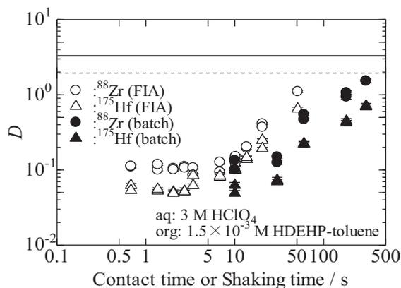
Fig. 2. Dependences of the  $D$  values of <sup>88</sup>Zr and <sup>175</sup>Hf on the contact time in the FIA apparatus or shaking time in the batch experiment. The dashed and solid line indicate the  $D$  values of <sup>88</sup>Zr and <sup>175</sup>Hf at equilibrium, respectively.
