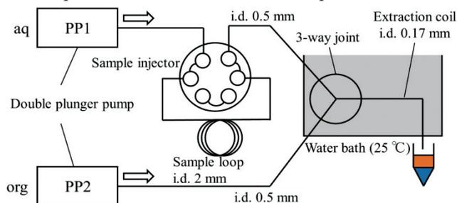
Fig. 1. Schematic view of the FIA apparatus setup.
