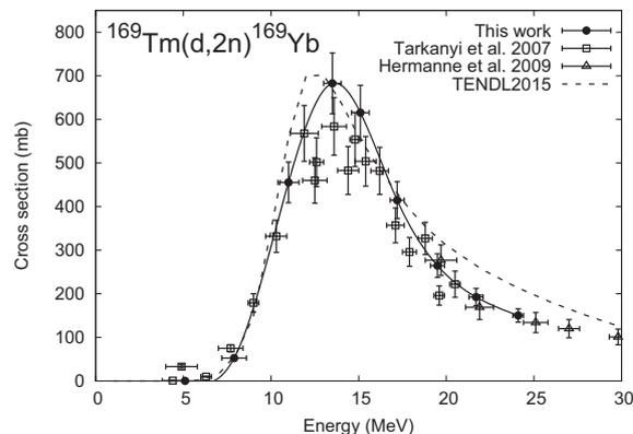
Fig. 1. The excitation function of the  $^{169}\text{Tm}(d,2n)^{169}\text{Yb}$  reaction is shown with a spline fit over our experimental data. The result is compared with the previous experimental data<sup>6-8)</sup> and TENDL-2015.<sup>12)</sup>
