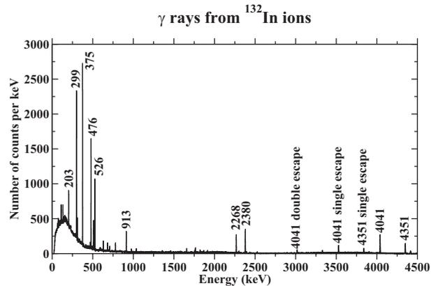
Fig. 1. Spectrum of  $\gamma$  rays obtained from the  $\beta$  decay of  $^{132}\text{In}$ . Strong previously reported decays are present<sup>4)</sup>.
