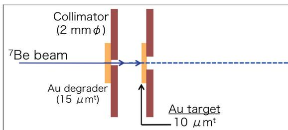
Fig. 1. Set up in the CRIB F2 chamber.
