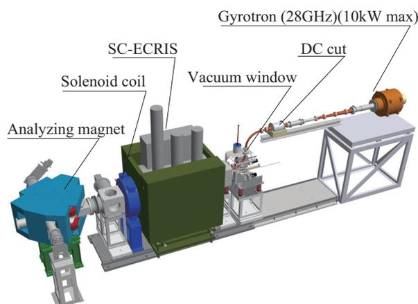
Fig. 2. Schematic drawing of the RIKEN 28 GHz SC-ECRIS.
