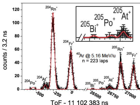
Fig. 4. Time-of-flight spectrum measured in the nuclear fusion reactions of  $^{169}\text{Tm}$  and  $^{40}\text{Ar}$ . Isotopes shown in the figure are clearly identified by comparison with tof-spectrum of a different number of flight laps,  $n = 224$ . RI of  $^{205}\text{Bi}$  was clearly identified within an error of 1  $\text{MeV}/c^2$  by two detected events, as shown in the inset.
