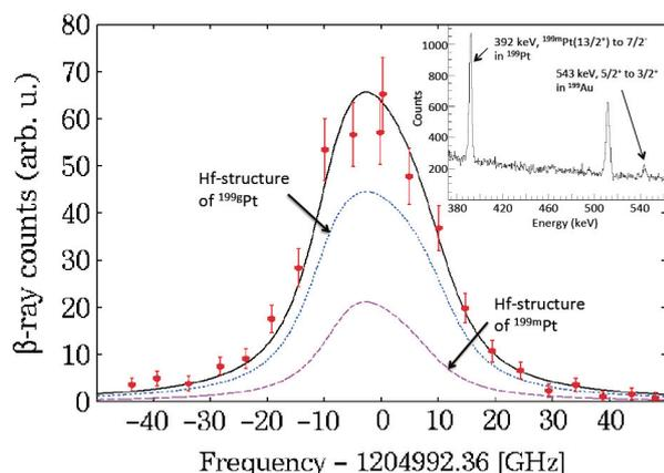
Fig. 3. Hyperfine (Hf-) structures of  $^{199m}, ^{199g}\text{Pt}$  obtained with  $\beta$ -transitions of  $^{199g}\text{Pt}$ . Short and long dotted lines indicate contributions of  $^{199g}\text{Pt}$  and  $^{199m}\text{Pt}$ , respectively. The Hf-structure of  $^{199m}\text{Pt}$  is independently determined by the internal  $\gamma$ -transition (392 keV) from  $^{199m}\text{Pt}$  shown in the inset.
