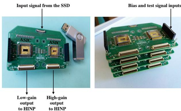
Fig. 1. Preamplifier boards for the GLAST silicon trackers. The left figure shows a single PCB. The right figure shows the assembly of the four PCBs into a compact stack.
