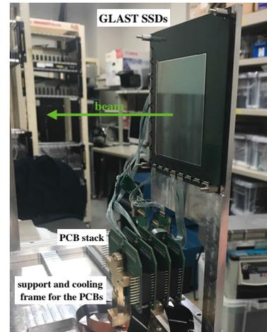
Fig. 2. Arrangement of the GLAST silicon detectors with preamplifier boards for the test experiment in HIMAC.
