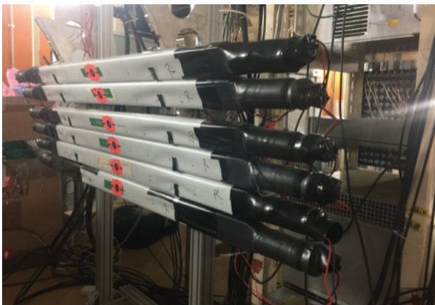
Fig. 1. Part of the VANDLE array setup at RIBF B3F. The delayed neutron will be detected by the array and the time-of-flight provides neutron energy.
