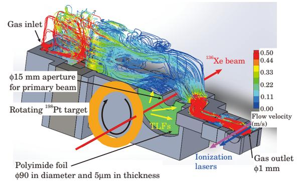
Fig. 1. Schematic view of the doughnut-shaped gas cell. The colored lines indicate the calculated argon gas flow trajectories connected to the gas outlet, based on the exact geometry. The color code indicates the calculated velocity (m/s) of the argon gas flow. Here, the pressure of the argon gas was 88 kPa.
