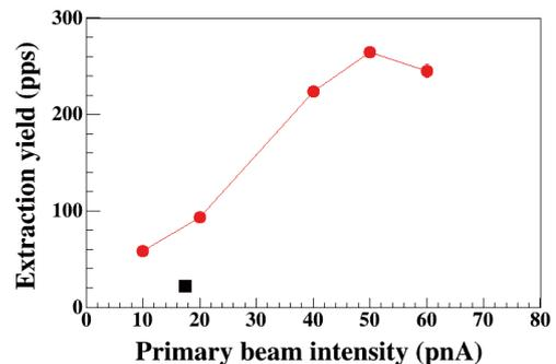
Fig. 2. Measured extraction yields as a function of primary beam intensity with the use of the old and new gas cells. Statistical error bars are smaller than the symbols.
