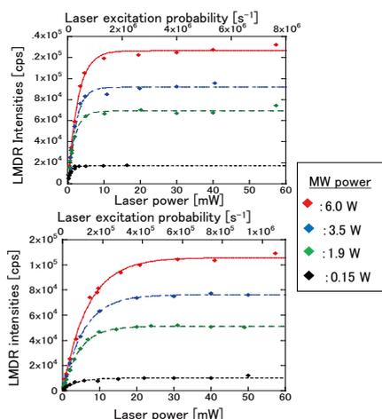
Fig. 1. Laser power dependence of LMDR intensities for different MW powers. The upper and lower figures show the result using Rb cells containing He buffer gas of  $1.3 \times 10^4$  Pa and  $1.0 \times 10^5$  Pa, respectively.
