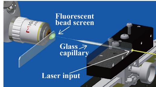
Fig. 1. Fluorescent beads,  $2 \mu\text{m}$  in diameter, shift the wavelength from 488 nm (input laser) to around 508 nm (fluorescence) in order to observe the spot shape at a specific distance.
