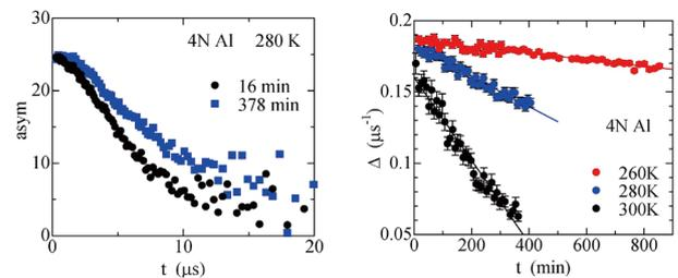
Fig. 1. (left) Zero-field muon spin relaxation spectra obtained for the pure Al sample at 280 K.
