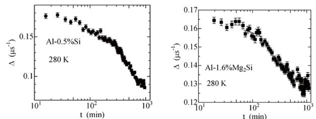
Fig. 3. (left) Time dependencies of dipole width in the Al-0.5 at.%Si alloy at 280 K.
