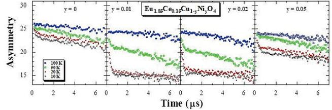
Fig. 1.  $\mu\text{SR}$  spectra of  $\text{Eu}_{1.85}\text{Ce}_{0.15}\text{Cu}_{1-y}\text{Ni}_y\text{O}_{4+\alpha-\delta}$  with  $y = 0, 0.01, 0.02,$  and  $0.05$  at various temperatures.<sup>5)</sup>
