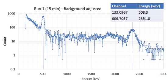
Fig. 3. An example of the  $\gamma$  ray spectra obtained for the “in-beam” measurement for the  $^{12}\text{C}(p,\gamma)^{13}\text{N}$  reaction with 2 MeV proton beams. The two  $\gamma$  ray peaks correspond respectively to the two low-lying resonances in  $^{13}\text{N}$ .
