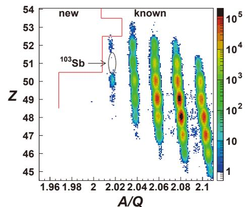
Fig. 2. The  $Z$  versus  $A/Q$  PID plot of the  $^{105}\text{Te}$  setting.
