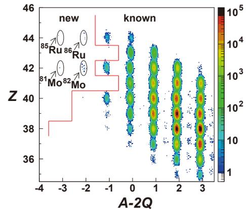
Fig. 1. The  $Z$  versus  $A - 2Q$  PID plot of the  $^{85}\text{Ru}$  setting. The fully stripped events ( $Z - Q = 0$ ) are selected. The solid lines indicate the limits of known isotopes as of June 2017.
