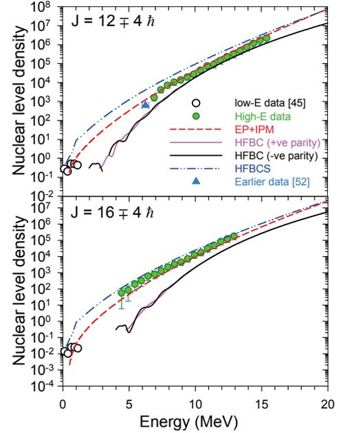
Fig. 1. Angular momentum gated NLD (symbols) along with the results of different theoretical calculations.
