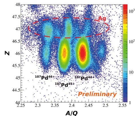
Fig. 2. Correlation of proton number  $Z$  and mass-to-charge ratio  $A/Q$  of reaction residues produced from a  $^{107}\text{Pd}$  beam at 32 MeV/nucleon and a  $\text{H}_2$  target.
