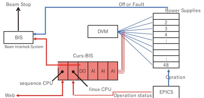
Fig. 1. Schematic diagram of the beam interlock system driven by change in current (Curs-BIS). The parts drawn in red are newly installed.
