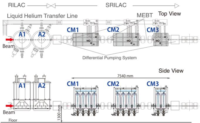
Fig. 1. Layout of the Superconducting RILAC (SRILAC).
