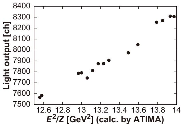
Fig. 1. Relation between light output from LaBr<sub>3</sub>(Ce) crystal and calculated  $\frac{E^2}{Z}$  by ATIMA.<sup>5)</sup>
