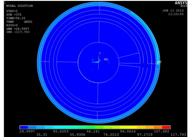
Fig. 2. A  $^{48}\text{Ca}$  primary beam at 345 MeV/nucleon with 470 pA (7.8 kW in beam power) onto the beryllium target of 10 mm thickness. The heat deposited in the target was 0.96 kW for a beam spot size with a diameter and rotation speed of 1 mm and 10 rpm, respectively. The maximum beam spot temperature is approximately 118°C.
