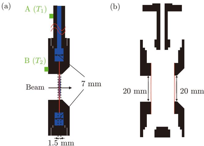
Fig. 1. (a) Side view of the cross-section of target cell. Blue area is filled with liquid hydrogen. Green squares indicate the thermometers. (b) Side view of the cross-section of target cell components.
